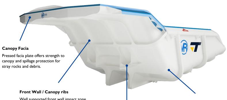
Well supported front wall impact zone with continuous ribs reinforcing the front wall to canopy joint and providing exceptional support to overhanging canopy. Structural strength reduces risk in event of roll over.
